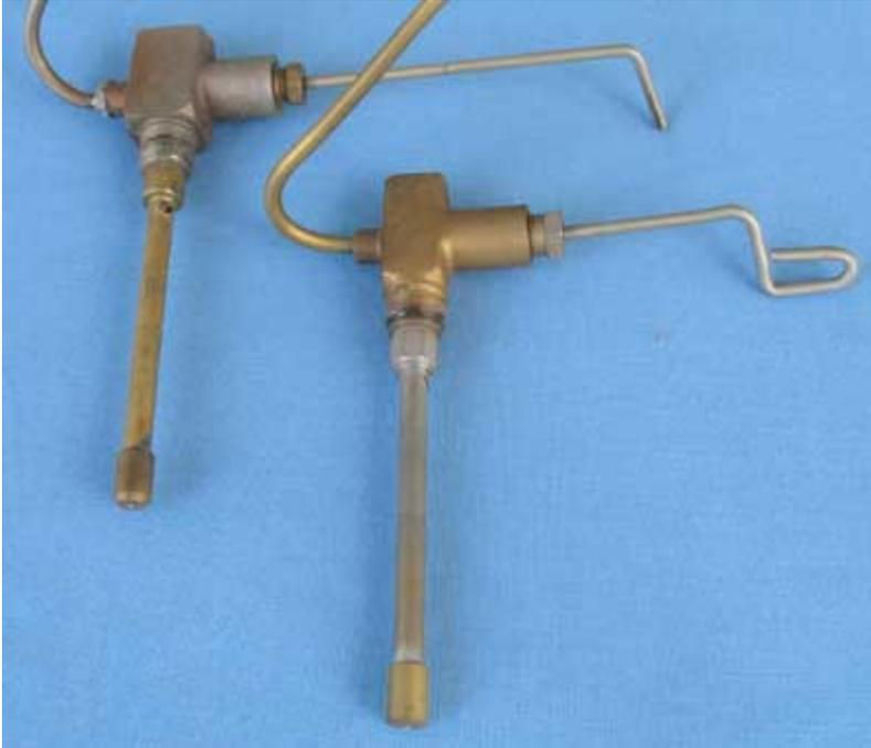
Figure 4. Fuel valve bodies from a Canadian 500 date-stamped C 38, left, and from a US 500 date-stamped B 41, right (Terry Marsh collection)
