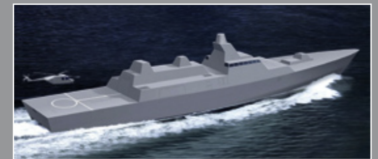
VISBY+ STEALTH CORVETTE Length 88,0 m · Beam 15,0 m · Draught 3,2 m · Displacement (full) 1 500 t Speed at full displ. 33 kn · Range at 14 kn: 3 000 nm · Endurance approx. 21 days
