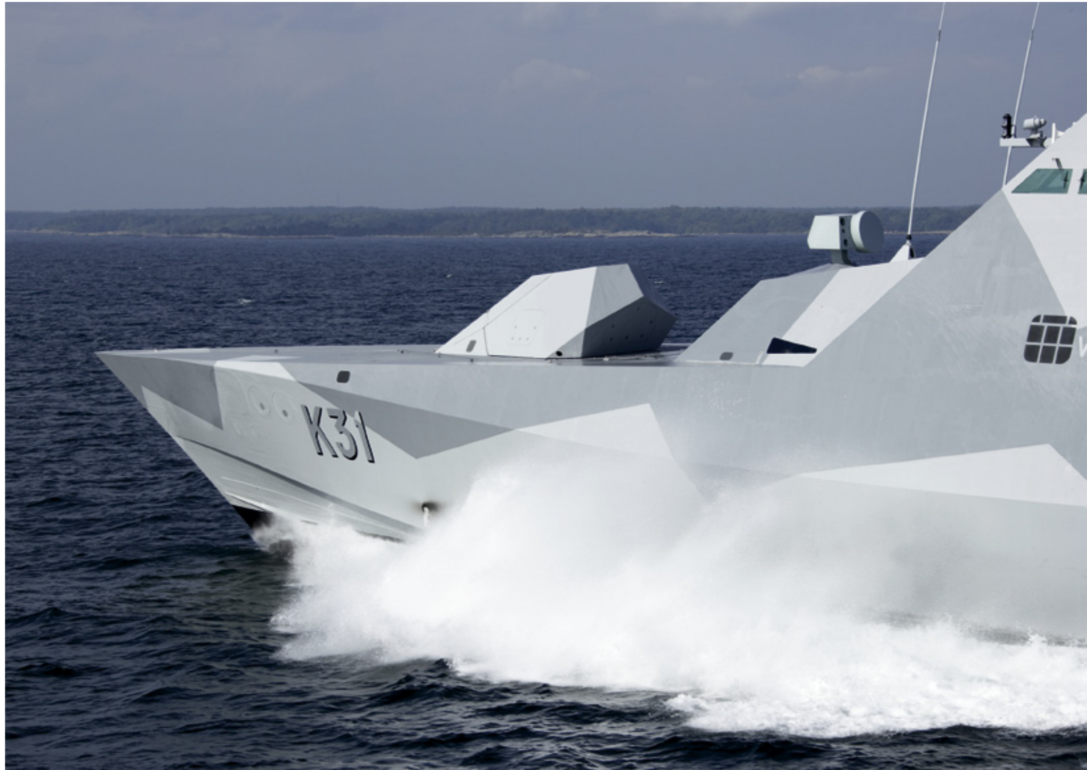
On Visby, great lengths have been taken to control the Radar Cross Section (RCS) signatures of all exterior items: Angled hull surfaces and special reduced reflecting coating systems, concealed weaponry and deck gear housings, non-reflecting window glass etc.
