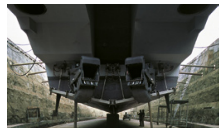
Gas turbines (top, left) and the encapsulated diesels (top, right), deliver power to the water jets as required (below)
