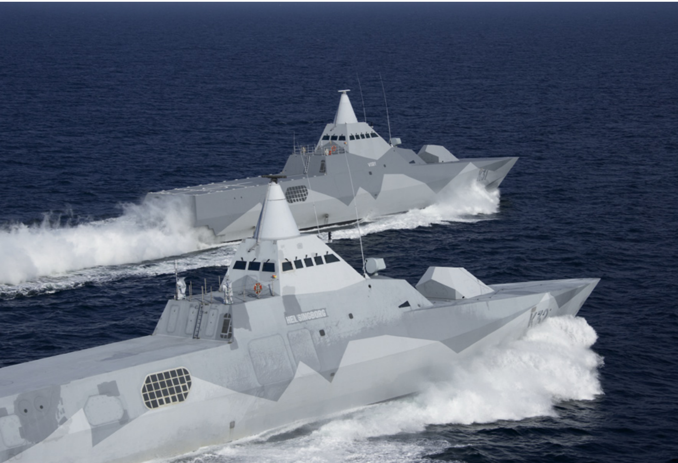
HELSINGBORG and VISBY at flank speed of 35+ knots. In order to render themselves detectable for Radar in friendly waters, both vessels have reflectors set astern of the bridges. The railings and life rings, detrimental to the RCS, are only rigged on non-hostile missions when maximum stealth is not of importance.
