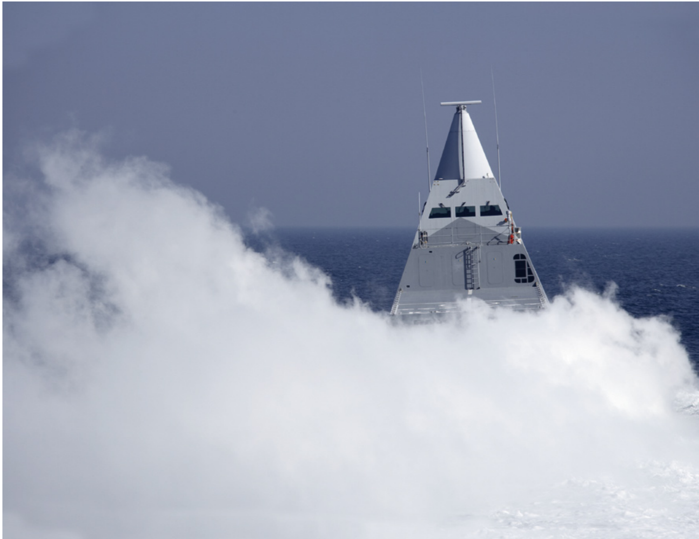
The vapour plume from diesel / gas turbine water cooled exhaust gases feigns the vessel's true location to infrared sensors on incoming threats.
