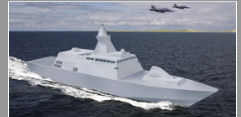
VISBY EXPORT STEALTH CORVETTE Length 68,3 m · Beam 12,3 m · Draught 2,4 m · Displacement (full) 650 t Speed at full displ. 35+ kn · Range at 15 kn: 2 500 nm · Endurance approx. 21 days
