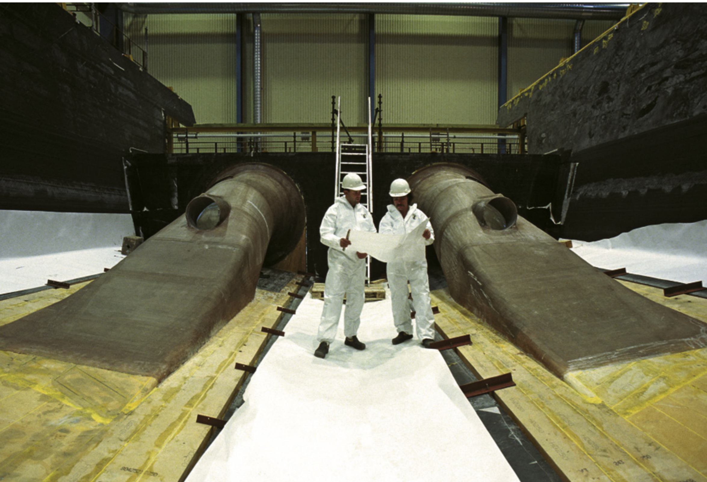
High-tech in Carbon fibre: Water jet intakes and ducts are bonded to the hull, as all longitudinals and bulkheads, and form a homogeneous structure of enormous rigidity.
