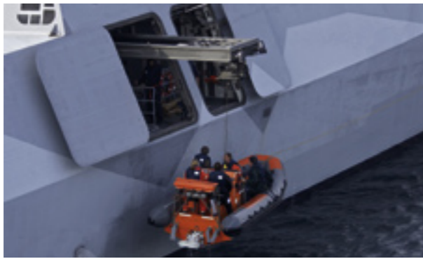
Visbys' boats, RIBs, ROVs etc. are stored behind flush fitting hanger doors, and launched from telescopic gantry cranes
