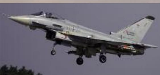
Development aircraft DA5 during the tests for the LERX - Leading Edge Root Extensions (marked in orange at join between the wing and the fuselage).
